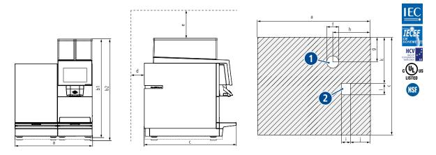
1 Cut-out for water/milk inlet and water drain. Also possible for power 2 Cut-out for grounds ejection.
