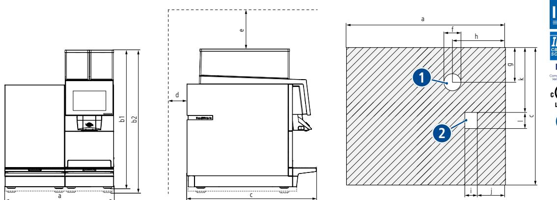
1 Cut-out for water/milk inlet and water drain. Also possible for power cord.
